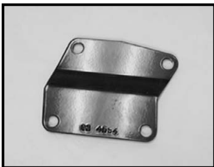
Part # 34100-03 / Qty. 1 DS front differential forward mount
