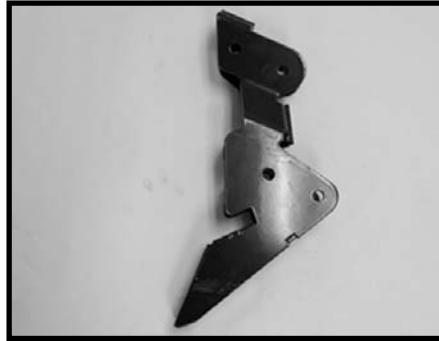
Part # 34100-13 / Qty. 1 DS rear lower control arm frame bracket
