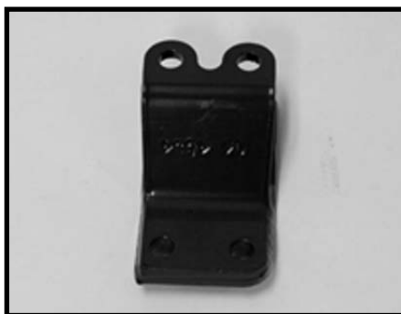
Part # 34100-04 / Qty. 1 PS front differential forward mount
