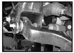
9. With both strut assemblies out of the vehicle it is time to 15. Working on the driver side, attach the sway bar back to of the stock strut cap and secure them using the stock nuts. passenger side and torque to 50 ft lbs. Torque to 35 ft lbs.
