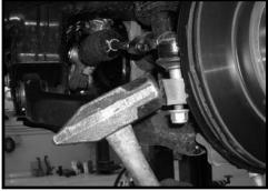
that the vehicle is stable and can't roll backwards. Safely lift 6. Working on the driver side, disconnect the sway bar end the front of the vehicle and support the vehicle with a pair of link from where it is connected to the sway bar, do not disjack stands. Place a jack stand on both the driver and the connect the end link from the lower control arm. Repeat on
