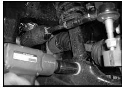
8. Working on the driver side, loosen but do not remove the (2) bolts holding the lower control arm to the vehicle. Repeat on passenger side. Special note: This is done so that the lower control arm can swing down and allow you to remove the strut assembly from the vehicle. Also, carefully use a pry bar to help remove the struts from the vehicle.
