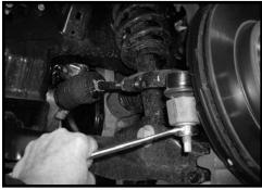
5. Now return to the upper ball joint and outer tie rod and carefully break the taper and remove them both from the steering knuckle. Repeat on passenger side. Special Note: Take special care not to damage the ball joint and tie rod end rubber boots.
