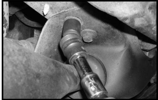
9. Locate the new front twin eye beam relocation bracket and the stock hardware. Install the new front relocation bracket to the stock location and secure using the stock hardware. Make sure to use thread locker or loctite and torque to **85 ft lbs.**
