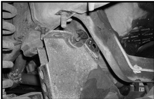
7. Working on the rear passenger side twin eye beam axle, remove the stock mounting hardware that connects the rear axle to the stock location. The stock hardware may be discarded.
