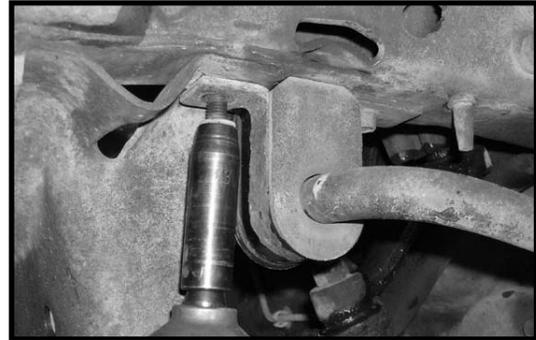
3. Working on the driver side, remove the stock sway bar end link from the stock axle location. Save the hardware. Repeat procedure on the passenger side. Set the sway bar aside.
