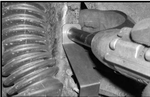
27. Locate (2) e-clips from hardware bag FBLNB2. Working on the driver side, install the new e-clips to the stock brake line on the back side of the newly installed brake line relocation bracket. Repeat procedure on the passenger side. **Special note: Once the installation of this suspension is completed and the weight of the vehicle is on the ground, check to make sure that the stock brake line does not rub on the inside of the tire.**
