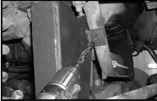
11. Locate (1) 1/2" x 1 1/2" bolts, (2) 7/16" USS flat washers and (1) 1/2" unitorque nuts from hardware bag R4NB. Secure the newly installed front axle pivot relocation bracket to the front cross member using the new 1/2" x 1 1/2" bolt and hardware. Make sure to use thread locker or loctite and torque to **75 ft lbs.**
