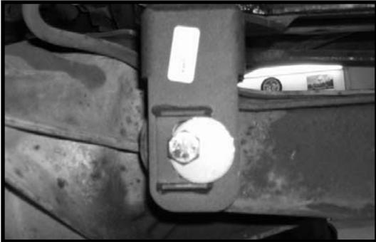
18. The brackets around the "D" bushings on the stock front sway bar may need to be opened up to 7/16". Try a 7/16" bolt in each location to make sure that it will fit. If not, open the holes up so that the new 7/16" bolts will fit.
