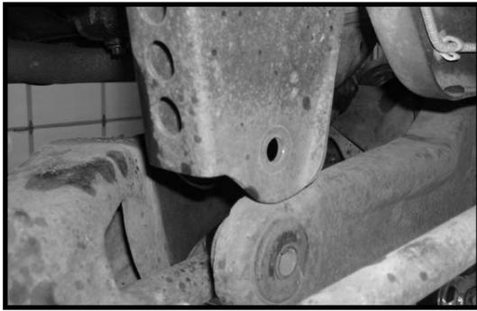
6. Working on the front driver side twin eye beam axle bracket, remove the stock bracket from the stock location. Save the stock hardware but the the stock bracket may be discarded.
