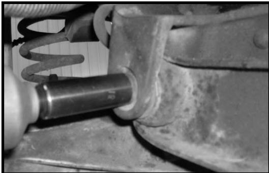
8. Working on the driver side stock radius arm bracket, remove the stock hardware or the stock rivets that connect the bracket to the frame rail. The stock hardware and rivets may be discard. Repeat procedure on the passenger side. **Special note: Using a die grinder and making a cross cut on the rivets then using a air chisel will help make the removal of the rivets easier.**
