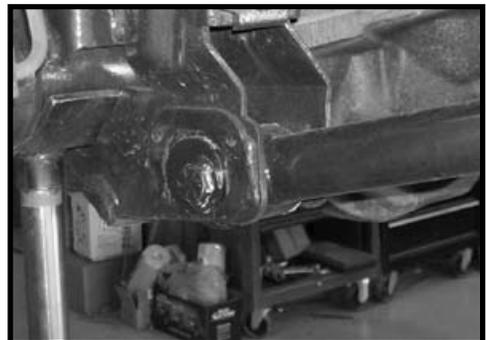
20. Locate (2) 9/16" x 4" bolt, (4) 1/2" USS flat washers and (2) 9/16" unitorque nut from hardware bag 30940NB1. Also, locate the new upper control arm. Working on the driver side, install the new upper control arm into the stock axle pocket
