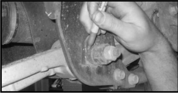
6. Working on the driver side, remove the hardware that attaches the lower control arm to the front and rear lower control arm mounts. Save the hardware. Repeat procedure on the passenger side. **Special note: Let the lower control arms hang and rest on the hydraulic floor jacks.**
