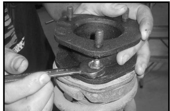
9. Locate (6) 3/8 nylon nuts and (6) 5/16" USS flat washers from hardware bag D2P-NB. Working on the driver side, install the newly modified coil over into the upper location and secure using the new hardware. Make sure to use loctite and torque to **32 ft lbs**. Repeat procedure on the passenger side.
