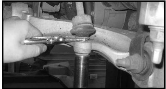
4. Working on the driver side, remove the hardware that attaches the coil over to the lower control arm. Save the hardware. Repeat procedure on the passenger side.
