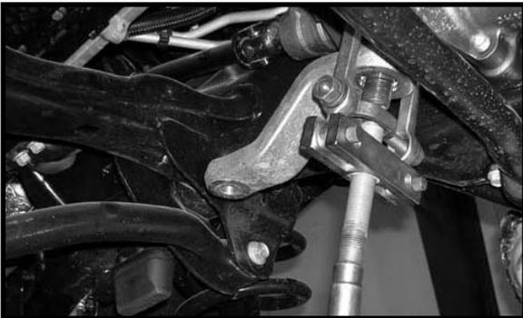
7. Locate the new pitman arm and the pitman arm hardware. Install the new pitman arm into the stock location on the sector shaft and secure using the stock hardware. Make sure to use loctite. Torque the nut on the sector shaft to **225 ft lbs.**
