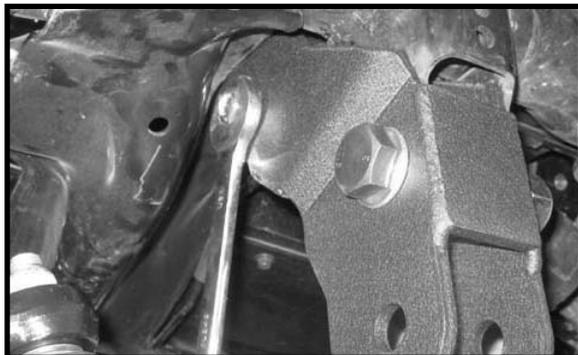
16. Move back to the 18 mm hardware attaching the new bracket to the OE location and add some loctite and torque to **95 ft lbs.**
