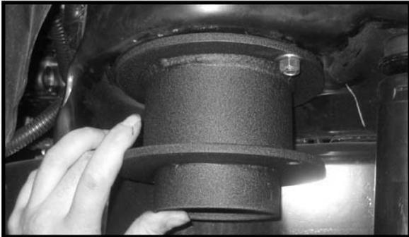
20. Locate the OE coil spring isolator. Working on the driver side, install the OE coil spring isolator to the newly installed coil spring spacer. **Special note: Make sure that the nipple of the isolator fits properly into the hole on the lower ring of the new coil spring spacer.** Repeat procedure on the passenger side.
