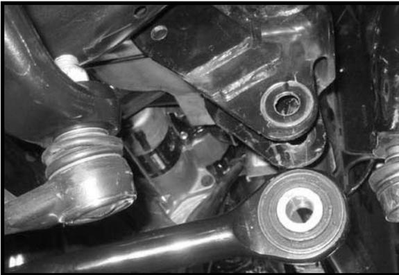
12. Working on the front portion of the OE track bar bracket, carefully enlarge the 3/8" hole to a 1/2" hole using a electric drill.
