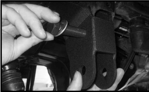
15. Move back to the 1/2" x 1 1/4" hardware attaching the new bracket to the OE bracket and add some loctite and torque to **38 ft lbs.**
