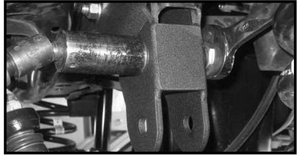
17. Install the track bar to the newly installed track bar bracket and secure using the OE hardware. Make sure to use loctite and torque to **145 ft lbs.** **Special note: If you are not able to install the track bar to the newly installed track bar bracket, this step will need to be performed when the suspension system is completely installed and the weight of the vehicle is on the ground.**
