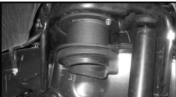
21. Locate the OE coil springs. Working on the driver side, install the coil spring back into the vehicle. Carefully raise up on the hydraulic floor jack until the coil spring seats properly into the newly installed isolator and coil spring spacer. Repeat procedure on the passenger side.
