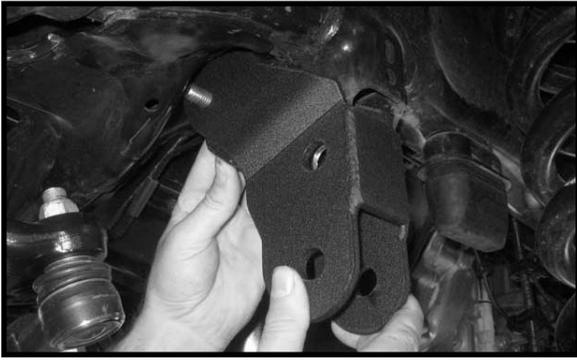
14. Locate the new S10242 sleeve. Also, locate (1) 18 mm x 90 mm bolt, (2) 18 mm flat washers and (1) 18 mm unitorque nut from hardware bag 33118NB. Using the new 18 mm bolt, hardware and sleeve, secure the new track bar relocation bracket to the stock track bar bracket OE hole. Do not tighten at this point. **Special note: The new sleeve will be installed inside the OE bracket.**
