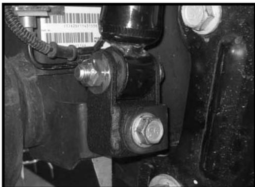
24. Working on the driver side, install the sway bar back to the sway bar end link and secure using the OE hardware. Make sure to use loctite and torque to **40 ft lbs**. Repeat procedure on the passenger side.
