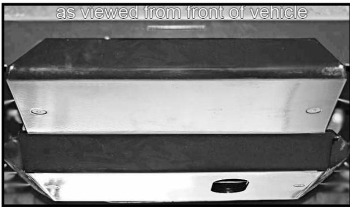
46. Working on the driver side add some thread locker or loctite to the hardware attaching the front and rear cross member to the frame mounts. Now torque this hardware to **75 ft. lbs.** Repeat procedure on the passenger side.
