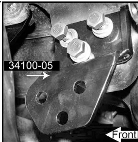
20. Locate the passenger side differential relocation bracket. Locate the passenger side differential stock bolts. Also, locate (4) 12 mm flat washers and (2) 12 mm unitorque nuts from hardware bag 34100NB8. Working on the passenger side, install the new passenger side differential relocation bracket to the frame using the stock bolts and new 12 mm hardware. **Do not tighten at this point.**
