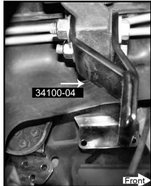
21. Working on the driver side of the removed front differential, disconnect the inner CV axle assembly from the differential. **Special note: Using pry bars, positioned between the inner CV and the differential will help free the axles.**
