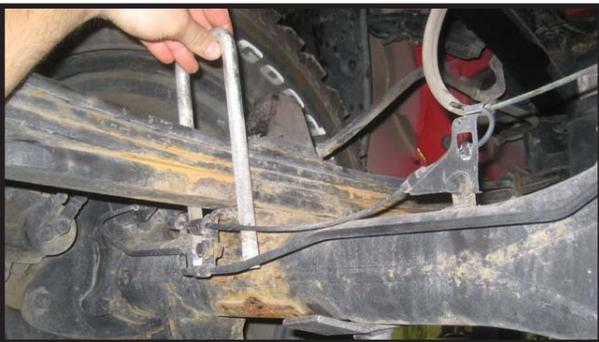
25. Carefully lower down on both hydraulic floor jacks at the same time allowing enough room for the rear blocks to be installed. **Special note: Take special care not to over extend any brake lines and/or hoses.**
