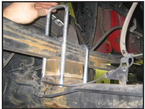
28. Reinstall the lower shock mounting locations using the OE hardware.
