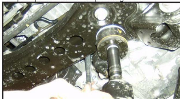
4. Locate (2) S10051 sleeves. Also, locate (2) 1/2" x 6" bolts, and (2) 1/2" unitorque nuts. Working on the driver side, install the new spacer between the differential and the OE mount and secure using the new 1/2" hardware, make sure to use the OE over size washer on the head side of the bolt. Repeat procedure on the passenger side. Move back to the new hardware hardware on the driver and passenger side and add some loctite and torque to **55 ft lbs.**
