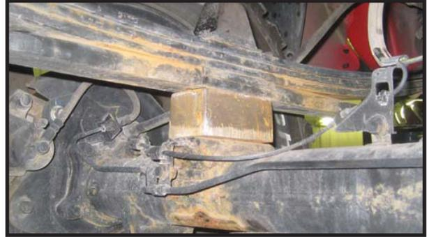
27. Locate (4) 9/16" x 2 9/16" x 9 5/8" square u-bolts. Locate (8) 9/16" u-bolt high nuts and (8) u-bolt washers from hardware bag 916NW. Also, locate the lower u-bolt plates. Working on the driver side, install the new u-bolts into the stock location and secure using the new 9/16" high nuts and washers. **Special note: If need be, cut off the excess threads off each leg of the newly installed u-bolts.** Torque to 120 ft lbs. Repeat procedure on passenger side.
