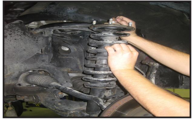
12. Locate the new upper strut spacers. Also locate the OE upper strut nuts that were removed in step #8. Install the strut spacers on top of the struts and secure using the OE nuts.
