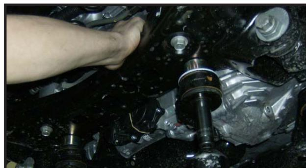
5. Place a pair of hydraulic floor jacks under the driver and passenger side lower control arm. Carefully raise up on them until they come into contact with the lower control arm. **You can do one side at a time if it works better for you.**
