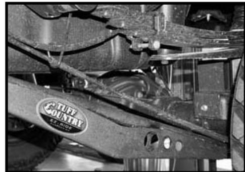
12. Carefully remove the hydraulic floor jacks from under the vehicle and carefully lower the vehicle to the ground. Once the weight of the vehicle is on the ground move back to the 1/2" x 3 1/2" bolts connecting the ladder bar to the new mounts and add some thread locker or loctite and torque to **65 ft lbs**.
