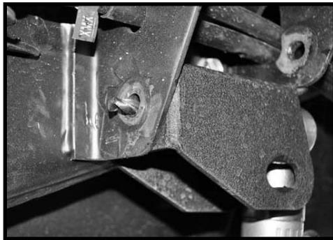
9. Locate (4) 1/2" x 1 1/4" bolts, (8) 7/16" USS flat washers and (4) 1/2" unitorque nuts from hardware bag 10892NB. Working on the driver side and using the new 1/2" hardware, secure the new front bracket to the previously drilled holes. Make sure to use thread locker or loctite and torque to **65 ft lbs**. Repeat procedure on the passenger side.
