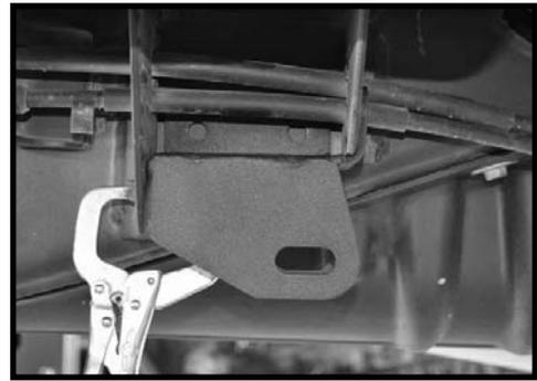
6. Using the new bracket as a guide, carefully drill (2) 5/16" holes into the frame rail. **Special note: Make sure to hold the the cables running through the body mount bracket away from the drill and take special care not to damage the cables.** Repeat procedure on the passenger side.
