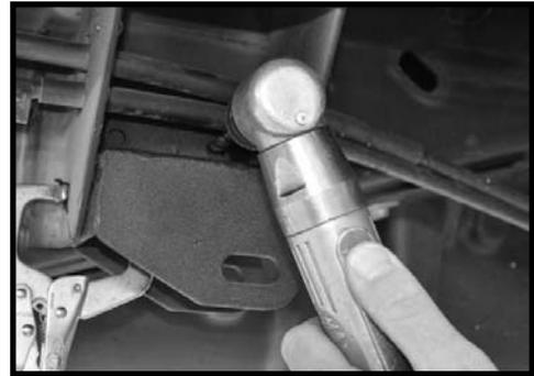
7. Locate (4) 3/8" x 1" self threading bolts from hardware bag 10892NB. Working on the driver side, secure the front driver side bracket to the frame rail using the new 3/8" x 1" self threading bolts. **Make sure to use thread locker or loctite.** Repeat procedure on the passenger side.
