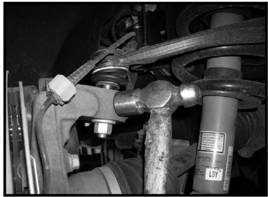
4. Working on the driver side, remove the hardware that connects the strut to the lower control arm. Save the hardware for later re-installation. Repeat procedure on the passenger side.
