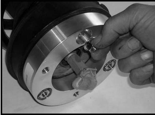
8. Locate the modified driver side strut. Also, locate (3) 7/16" x 1" bolts, (3) 3/8" USS flat washers and (3) 7/16" lock washers from hardware bag 12000NB. Install the modified driver side strut into the **PASSENGER** side upper location and secure using the new 7/16" x 1" bolts and hardware. **Do not tighten at this point.**
