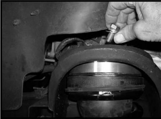
9. Locate the modified passenger side strut. Also, locate (3) 7/16" x 1" bolts, (3) 3/8" USS flat washers and (3) 7/16" lock washers from hardware bag 12000NB. Install the modified passenger side strut into the **DRIVER** side upper location and secure using the new 7/16" x 1" bolts and hardware. **Do not tighten at this point.**
