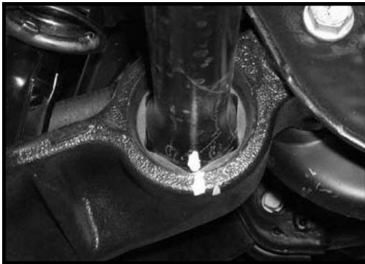
4. Working on the driver side and using a proper torsion bar removal tool. **Special note: Tuff Country EZ-Ride Suspension requires that a proper torsion bar unloading tool be used when performing this installation. If you do not have one, please contact your local GM dealer to purchase one from them.** Carefully remove the stock torsion bar bolt and block. Set the stock torsion bar bolt and block aside. Remove the stock torsion bar unloading tool from the stock cross member.
