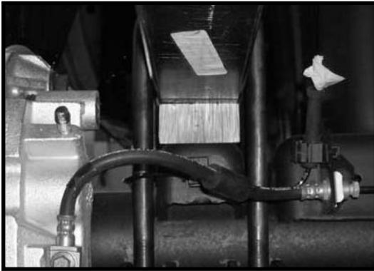
18. Working on the driver side, install the stock shock back into the axle mount using the stock hardware. Make sure to use thread locker or loctite and torque to **75 ft lbs.** Repeat procedure on the passenger side.
