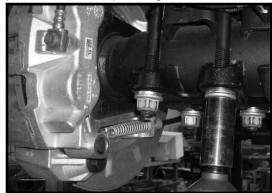
14. Carefully lower down on both hydraulic floor jacks at the same time approximately 2". **Special note: Take special care not to over extend any brake lines and/or hoses.**
