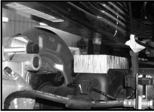
16. Carefully raise up on both hydraulic floor jacks at the same time until the stock spring assembly sits flush with the newly installed 1" lifted block.
