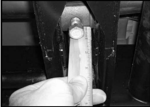
**Special note: If the stock torsion bar bolt is over adjusted, ride quality issues will occur and over adjusting the bolt is not recommended.**
