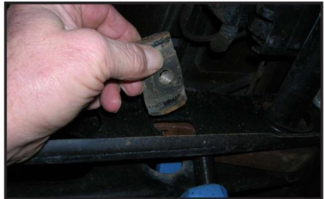
5. Working on the driver side, tap the torsion bar forward until the torsion bar key can be removed.
