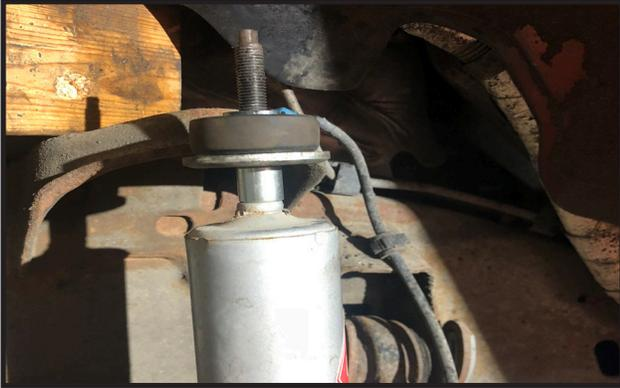
10. Re-install the OE shock using the OE bushings and hardware.
