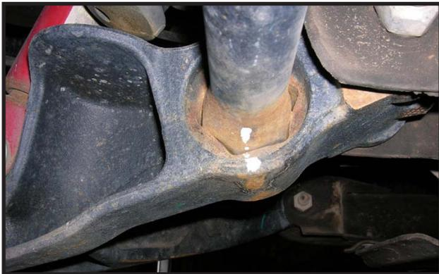
4. Working on the driver side and using a proper torsion bar removal tool. **Special note: Tuff Country EZ-Ride Suspension requires that a proper torsion bar unloading tool be used when performing this installation. If you do not have one, please contact your local GM dealer to purchase one from them.** Carefully remove the stock torsion bar bolt and block, and set aside. Remove the torsion bar unloading tool from the crossmember.
