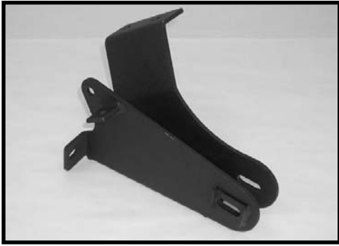
R401 / Qty. 1 Front axle pivot relocation bracket / (large)
