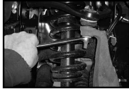
4. Working on the driver side, loosen but do not remove the nut from the outer tie rod. Repeat procedure on the passenger side.
