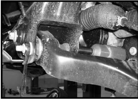
9. With both strut assemblies out of the vehicle it is time to install the new leveling spacers. Install these directly on top of the stock strut plate and secure them using the stock nuts. Torque to **35 ft lbs**.
