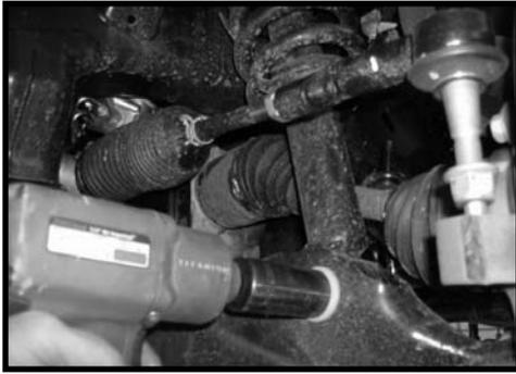
8. Working on the driver side, loosen but do not remove the (2) bolts holding the lower control arm to the vehicle. Repeat on passenger side. **Special note: This is done so that the lower control arm can swing down and allow you to remove the strut assembly from the vehicle. Also, the use of a pry bar may make removal easier.**
