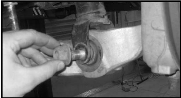
11. Working on the driver side, install the lower control arm into the front and rear lower control arm pockets using the OE hardware. Make sure to use loctite, refer back to the marks that were scribed on the cam washer and cam stops and torque the front and rear mounting hardware to **105 ft lbs**. Repeat procedure on the passenger side.
