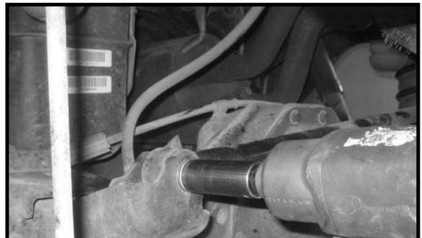
26. Working on the driver side, install the end link to the sway bar and secure using the OE hardware. Make sure to use loctite and torque to **40 ft lbs**. Repeat procedure on the passenger side.
