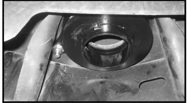
24. Working on the driver side, install the coil spring back into the OE location. Make sure that the OE rubber isolator is installed with the coil spring. Carefully raise up on the hydraulic floor jack until the coil spring seats properly into the lower axle. Repeat procedure on the passenger side.
