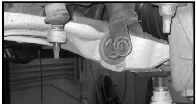
5. Working on the driver side, place a reference mark on the cam washer and cam stops that attach the lower control arm to the front and rear lower control arm mounts. Repeat procedure on the passenger side.
