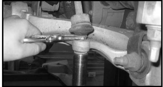
4. Working on the driver side, remove the hardware that attaches the coil over to the lower control arm. Save the hardware. Repeat procedure on the passenger side.
