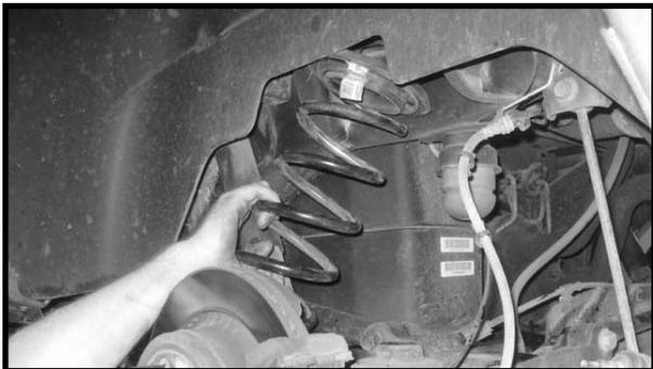
23. Locate the new rear coil springs spacers. Also, locate (2) 7/16" x 1 1/2" bolts, (4) 3/8" USS flat washers and (2) 7/16" unitorque nuts from hardware bag 32102NB. Working on the driver side, install the new 7/16" bolt into the upper coil spring bucket. Hole provided. Then install the new rear coil springs spacer into the upper coil spring bucket and secure using the new hardware. Make sure to use loctite and torque to **42 ft lbs**. Repeat procedure on the passenger side.
