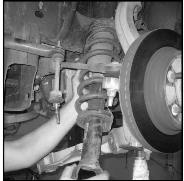
8. Install the new front spacers on the coil overs using the OE hardware. Make sure to use loctite and torque to **32 ft lbs.**
