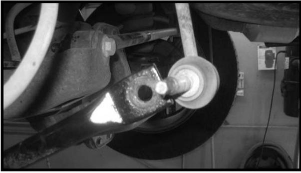
21. Working on the driver side, remove the track bar from the track bar location. Save the hardware.
