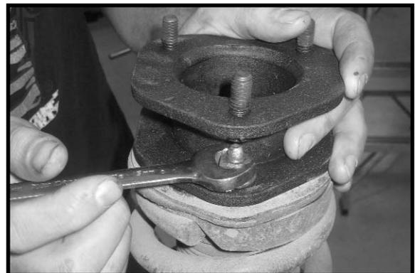
9. Locate (6) 3/8 nylon nuts and (6) 5/16" USS flat washers from hardware bag D2P-NB. Working on the driver side, install the newly modified coil over into the upper location and secure using the new hardware. Make sure to use loctite and torque to **32 ft lbs**. Repeat procedure on the passenger side.
