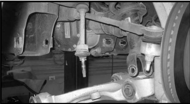
7. Working on the driver side, remove the (3) nuts that attach the coil over into the upper location. Save the hardware. Remove and set the coil over aside. Repeat procedure on the passenger side.
