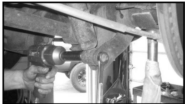
20. Working on the driver side, remove the sway bar end link from the sway bar. Save the hardware and repeat procedure on the passenger side.
