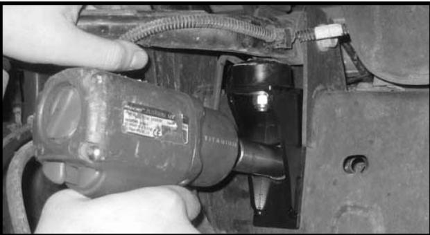
14. Locate the (2) zip ties in hardware bag 32102NB. Working on the driver side, zip tie the ABS line to the upper control arm so that ABS line does not get pinched between the upper control arm and the newly installed bump stop bracket. Repeat procedure on the passenger side.
