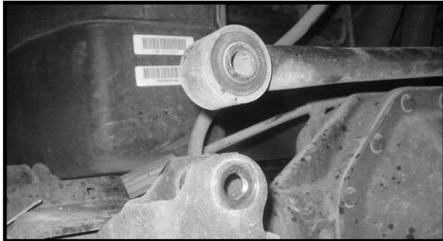
22. Carefully lower down on both hydraulic floor jacks allowing enough room for the rear coil spring to be removed. Working on the driver side, remove the rear coil spring and set aside. Repeat procedure on the passenger side.
