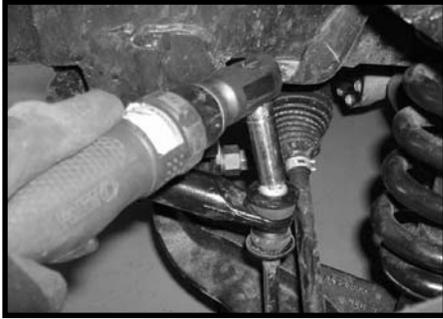
17. Move back to the stock outer tie rod that connects to the knuckle and torque to **65 ft. lbs.**
