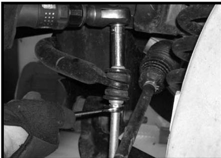
3. Working on the driver side, remove the stock outer tie rod nut that connects the tie rod to the knuckle. Save the stock hardware.
