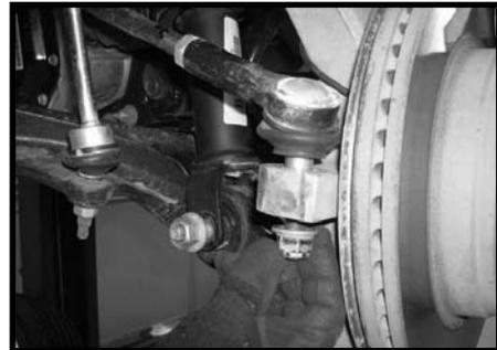
13. Locate the stock upper control arm hardware and working on the driver side, connect the stock upper control arm to the knuckle. **Do not tighten at this point.** Also, at this time, connect the ABS line to the stock clip on the back side of the knuckle.
