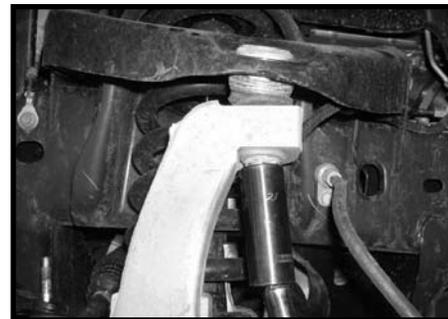
6. Working on the driver side, remove the upper control arm from the knuckle. Let the knuckle hang. **Special note: make sure not to over extended any brake hose and or wires.**
