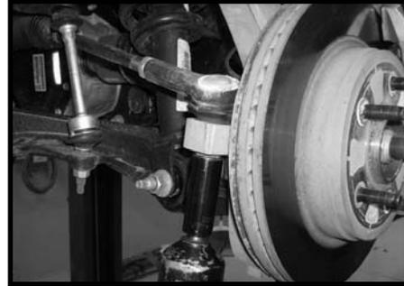
4. Working on the driver side, remove the stock outer tie rod from the stock knuckle.
