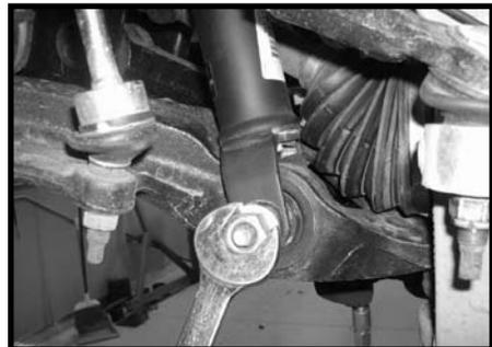
15. Working on the driver side new upper strut hardware add some thread locker or lock tite and torque all (3) nuts to **45 ft lbs.**
