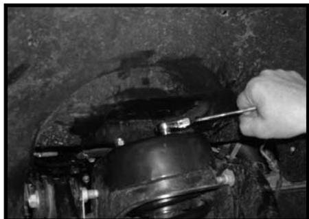
16. Locate the stock sway bar end link hardware and secure to stock sway bar to the stock end link. Add some thread locker or lock tite and torque to **32 ft lbs.**
