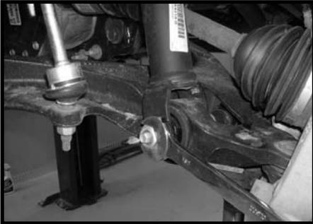
10. Locate (1) new strut spacer and the stock hardware that connected the stock strut into the stock location. Install the new spacer on top of the stock strut and secure using the stock hardware. **Make sure to use thread locker or lock tite and torque to 45 ft lbs.**
