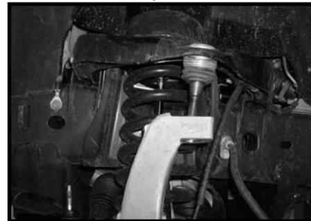
7. Working on the driver side, remove the stock ABS line from the stock clip on the backside of the stock knuckle.
