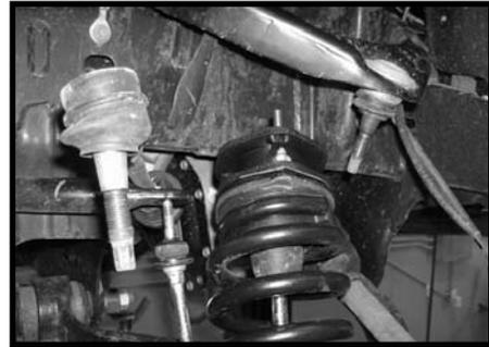
12. Locate the stock outer tie rod hardware and working on the driver side, connect the outer tie rod to the knuckle. **Do not tighten at this point.**
