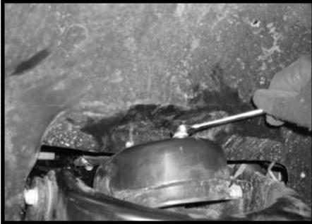
9. Working on the driver side, remove and save the stock hardware that connects the stock strut to the stock lower control arm. Set the stock strut aside.
