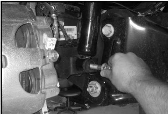
4. Working on the driver side, remove the sway bar end link from the sway bar. Save the hardware. Repeat procedure on the passenger side.
