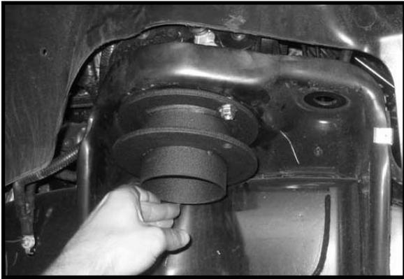
9. Locate the OE upper coil spring isolator and coil springs. Working on the driver side, install the isolator to the top of the coil spring and install the coil spring back into the vehicle. Carefully raise up on the hydraulic floor jack until the coil spring and isolator seat properly into the newly installed coil spring spacer. Repeat procedure on the passenger side.
