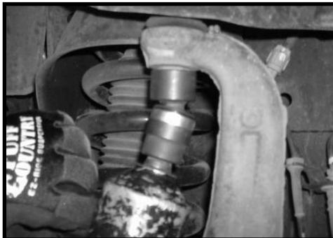
4. Working the driver side, carefully break the stock taper on the stock upper control arm and the stock knuckle. **Special note: Carefully hitting the stock knuckle with a hammer will help break the stock taper. Take special care not to damage the stock upper ball joint boot.** Do not remove the stock nut at this point. Repeat the procedure on the passenger side.
