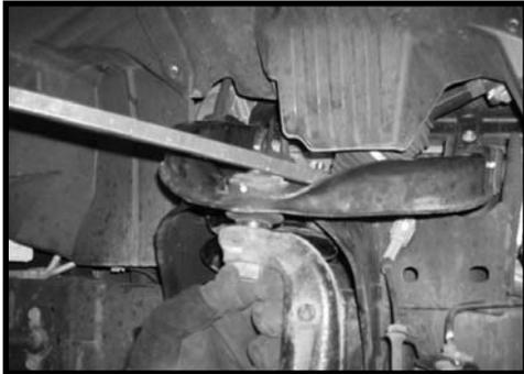
16. Working on the driver side, torque the stock upper control arm nut to **95 ft lbs.** Repeat procedure on the passenger side.
