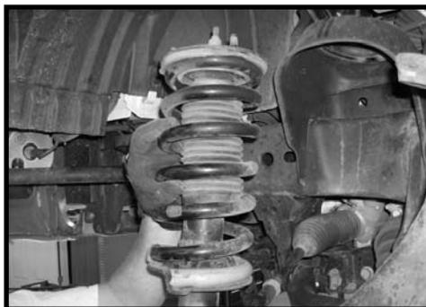
11. Locate the new strut spacers and the stock hardware. Working on the driver side strut, install the new spacer on top of the stock strut and secure using the stock hardware. Make sure to use thread locker or loctite and torque to **48 ft lbs.** Repeat procedure on the passenger side strut.
