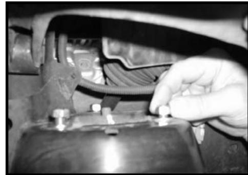
13. Locate the stock lower strut mounting hardware. Working on the driver side, secure the stock strut to the stock lower location and secure using the stock hardware. Make sure to use thread locker or loctite and torque to **95 ft lbs.** Repeat procedure on the passenger side.
