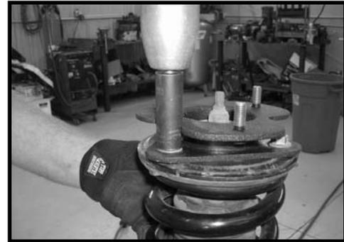
12. Locate (6) 3/8" nylon lock nuts and (6) 5/16" USS flat washers from hardware bag D2P-NB. Working on the driver side, install the modified passenger side strut into the stock upper driver side location and secure using the new 3/8" hardware. **Do not tighten at this point.** Repeat procedure on the passenger side with the driver side strut.
