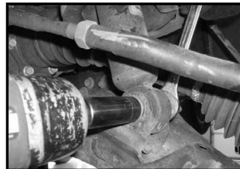
14. Locate the stock lower sway bar end link hardware. Working on the driver side, install the stock end link into the stock location and secure using the stock hardware. Make sure to use thread locker or loctite and torque to **42 ft lbs.** Repeat procedure on the passenger side.
