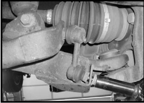
15. Locate the stock upper control arm mounting hardware. Working on the driver side, attach the stock upper control arm to the stock knuckle and secure using the stock nut. **Special note: A cheater bar may be needed to pull the upper control arm down so that it can be attached to the stock knuckle.** Repeat procedure on the passenger side.
