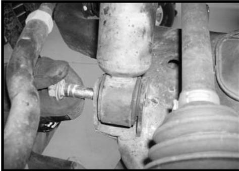
9. Working on the driver side, move back to the stock nut holding the stock upper control arm to the stock knuckle and remove. Save the stock hardware. Repeat procedure on the passenger side.
