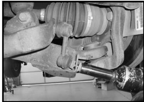
6. Working on the driver side, make a reference marking the driver side strut. Repeat procedure on the passenger side. **Special note: This is done because once the new spacers are installed on top of the stock struts, the driver side strut is going to be installed on the passenger side and the passenger side strut is going to be installed on the driver side.**
