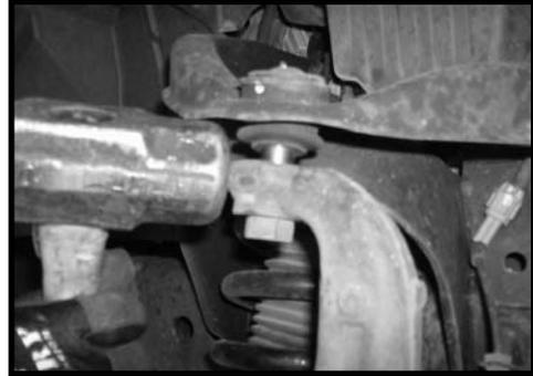
5. Working on the driver side, remove the stock lower sway bar end link hardware. Set the stock hardware aside. Remove the stock end link from the stock lower control arm. Repeat procedure on the passenger side.
