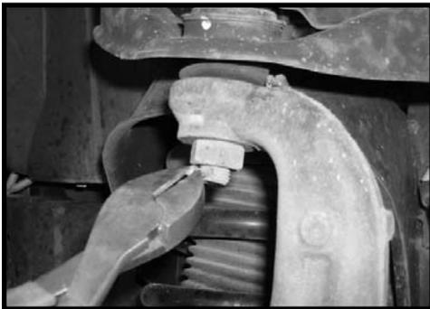
3. Working on the driver side, loosen but do not remove the stock nut connecting the stock upper ball joint to the stock knuckle. Repeat procedure on the passenger side.
